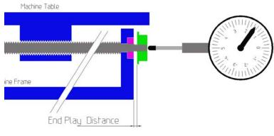
Endplay can be eliminated for the most part by a slight preloading of the thrust bearings. Take care not to preload the bearings too much as that may cause excessive drag, heating and premature wear of the thrust
