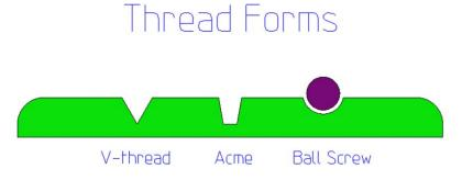
efficiencies of 30%. On a large machine this can be a significant loss of power on the axis. For small bench-top machines, V-thread losses are a small portion of a small expenditure of energy. The thread
