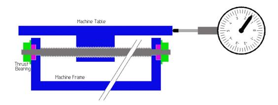
The same measurement can be made on a CNC machine by using the incremental jog, set to .001 inch increments. Jog the machine in a plus direction to move the indicator off zero. Then jog in the opposite
