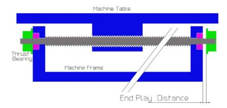
Typically the ends of lead screws will be machined to a precision diameter with shoulders and placed in a sleeve or ball bearing (thrust bearings). If the machine design does not have thrust bearings, or adjustment for endplay, changes in direction will result in a rotation of the screw without any corresponding motion of the slide.
